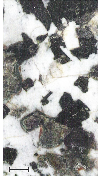
Gabbro with preserved igneous mineral stock. Augite black, Saussuritized plagioclase white.
