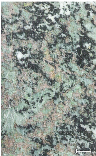
Eclogite metagabbro with the two Eclogite minerals garnet and omphacite, plus black Mg chloride and white zoisite.
